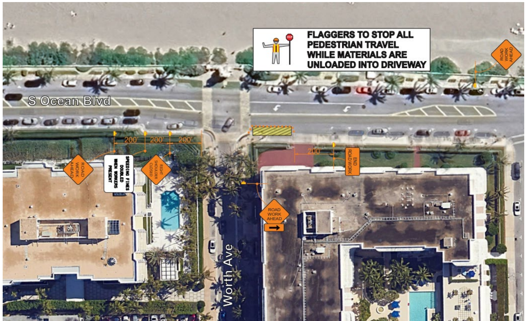
Figure 1 - 100 Worth Avenue Maintenance of Traffic Impacts on South Ocean Boulevard.
