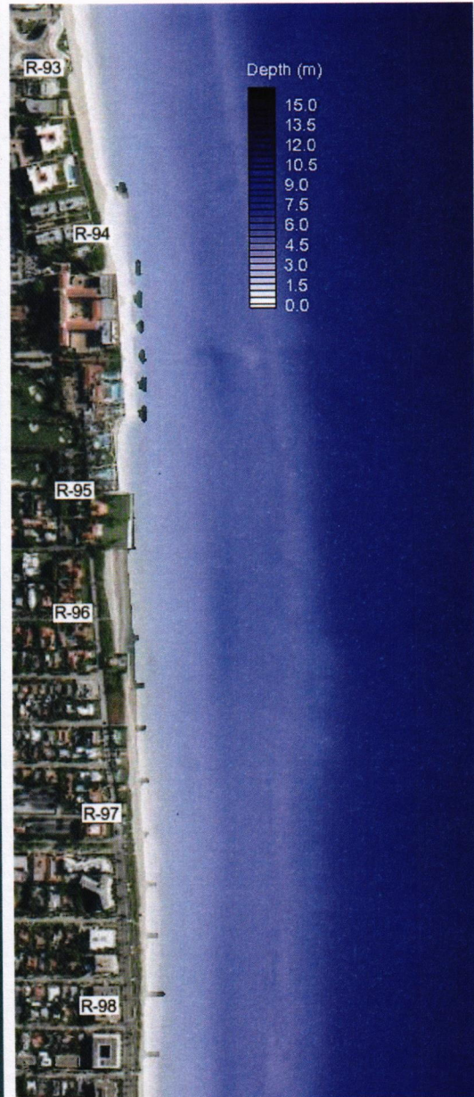
Figure 6. Model-Predicted Shoreline 2 Years Post- Project (Alternative 3).
