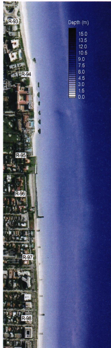
Figure 8. Model-Predicted Shoreline 2 Years Post-Project (Alternative 4).
