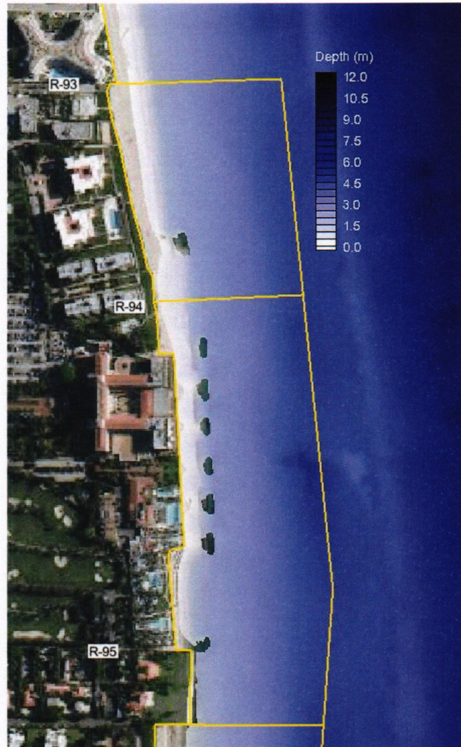
Figure 4. Model-Predicted Shoreline 2 Years Post-Project (Alternative 2).
