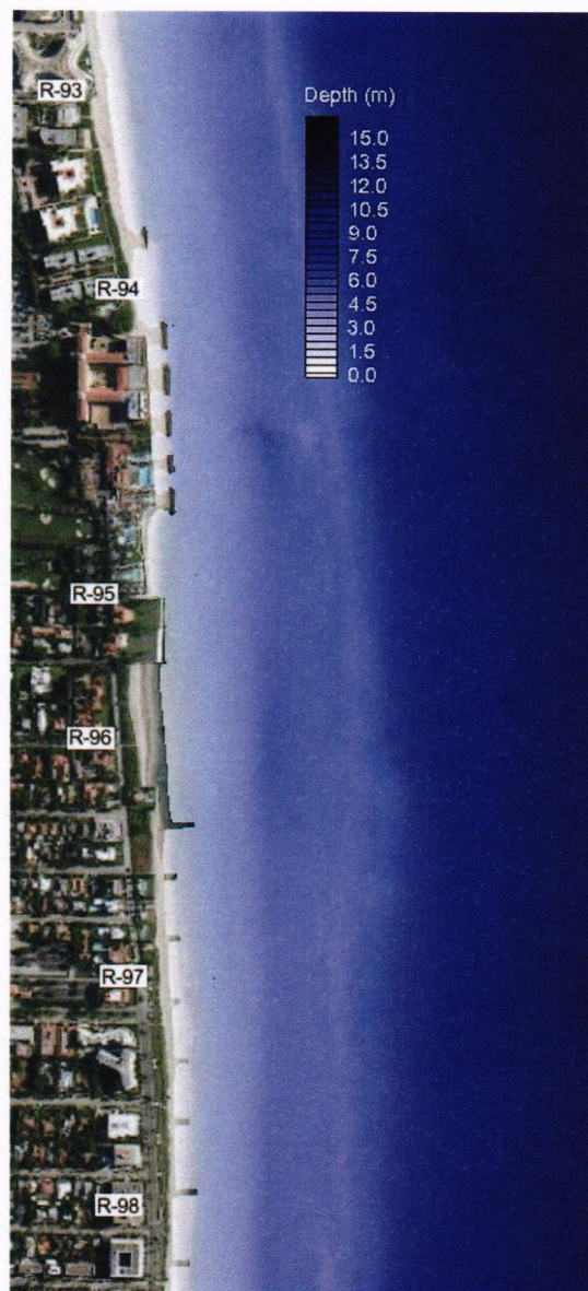
Figure 12. Model-Predicted Shoreline 2 Years Post-Project (Alternative 6).
